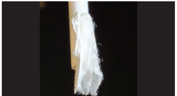
CollectEject Oral Swab showing cotton layers
